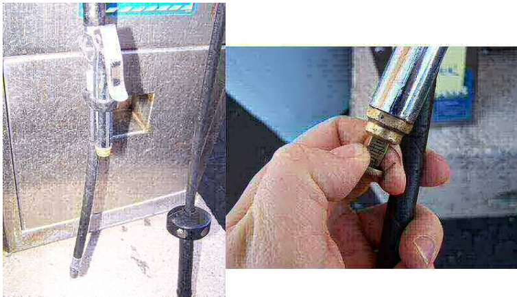
Air dispensing hose at a gas station with built-in pressure gauge
