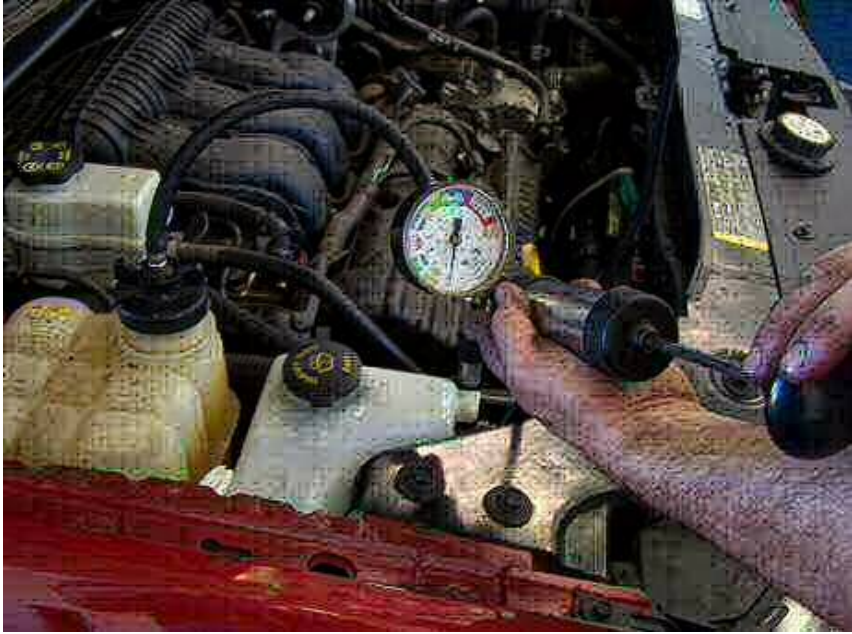
Pressure testing the cooling system
