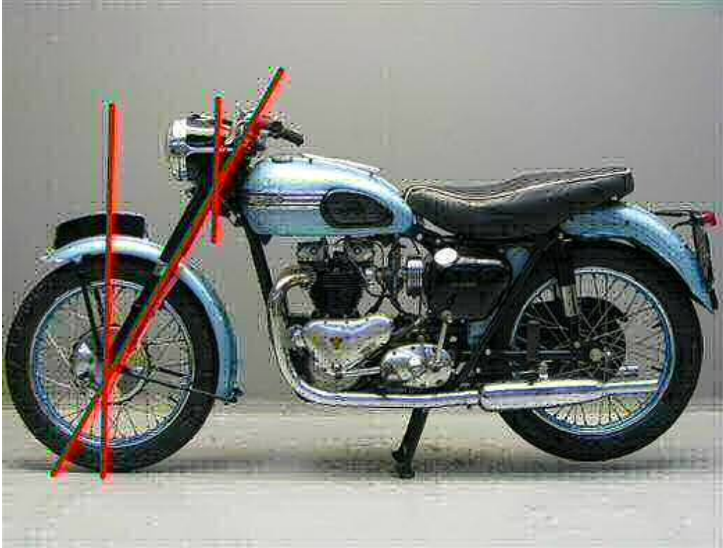
A positive caster is easily seen on the front wheels of motorcycles and bicycles. Image adapted, original credit: CC-BY-SA-Yesterdays Antique Motorcycles on Wikipedia
