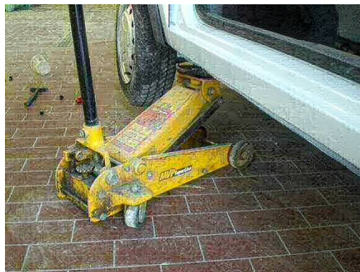
Hydraulic jack with hand-pump mechanism
