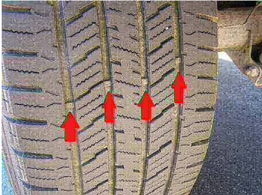
Tire with arrows pointing to the wear bars between the treads.
